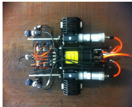
Figure 2: TOFD multi probe Inspection head on MAG-Rover.
