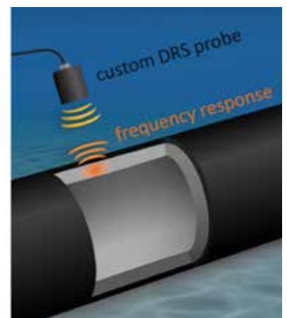
Figure 1. Dynamic Response Spectroscopy excites the coated pipe with ultrasonic energy and utilises the natural frequency response of the steel to determine its thickness.
