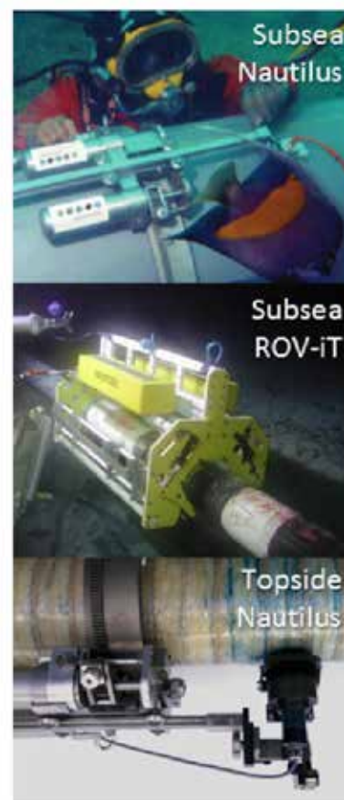
Figure 6. Sonomatic topside and subsea tools used for deployment of the DRS corrosion mapping technique.
