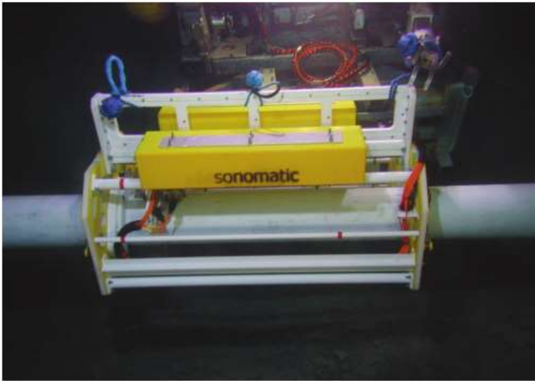
Figure 1. Inspection carried out using the ROV-IT, an ROV-deployed ultrasonic inspection tool developed by Sonomatic.
