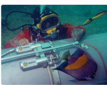
it can be used to inspect various components for pipewall corrosion mapping, pipe weld inspection, flange weld inspection, complex geometry welds (nozzle hop tap welds), and pipe ovality inspections (including measurements of surface dents). The system provides precise positioning and movement of transducers through a rigid, hinged collar attached to the component. It has a low profile design, allowing for a minimum clearance of 120 mm from the component surface.
