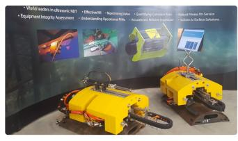
On the other hand, this unit is ROV deployed that harnesses power and data communication feeds from the ROV, making it a versatile system. Similar to the diver deployed system, it is interfaced with a Sonomatic Microplus digital ultrasonic imaging system and offers a wide range of ultrasonic inspection techniques including corrosion mapping, pulse-echo angle shear wave/phased array, time of flight diffraction (TOFD) and ACFM.
