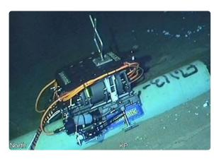
Sonomatic's Subsea MAG-ST crawler has been utilised for both subsea and topside applications and is deployed by an ROV onto the region of interest. The crawler is fixed to the pipe using permanent magnetic wheels, and its position can be recorded by onboard encoders and inclinometers to record positional feedback, whilst progress can be monitored using attached cameras.
