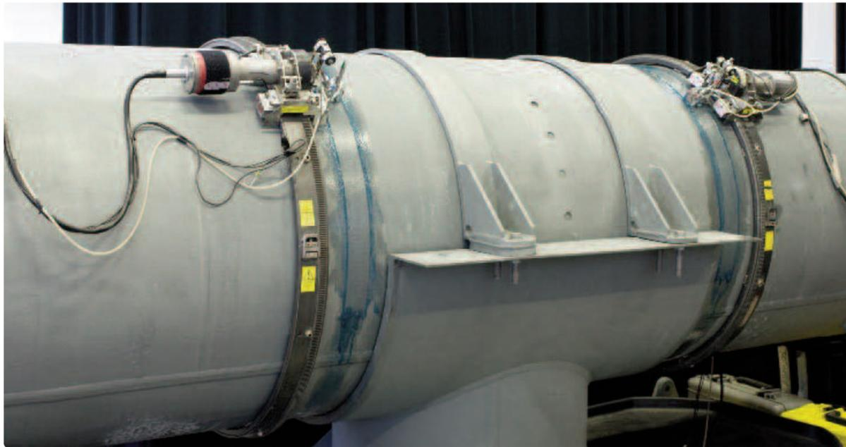
The Multiskip technique uses angled shear waves with two transducers in a pitch-catch mode. The transmitter and receiver can be separated by up to 2 m with full investigation of the material condition between the probes. The data can be collected while scanning at reasonably high speeds, allowing for rapid coverage of large areas.
