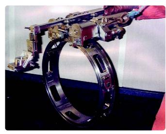
The Nautilus system facilitates very precise positioning and movement of the transducers via a rigid, hinged, collar attached to the component by saturation or air divers and is pressure rated to water depths of 250m. The collar provides a stable platform for the dual or triple axis, finely geared encoded scanner. The transducers can be moved in increments down to 1mm (or smaller) both circumferentially and axially around the component taking measurements at every location.
