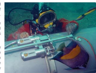
The manipulator is very adaptable and can be deployed in various formats to inspect a wide range of components for pipewall corrosion mapping, pipe weld inspection, flange weld inspection, complex geometry welds (nozzle HotTap welds) and pipe ovality inspections (including measurements of surface dents).
