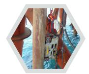
The marinised MEC<sup>™</sup>-MPS200+ Scanner supports the internal and external splash zone inspection of risers, flexible risers, caissons, conductors and structures with wall thickness up to 1″ and through coating of up to 15mm Neoprene and 4mm Monel clad.
