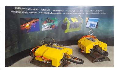
inspections techniques can be deployed, including Corrosion Mapping, Pulse-Echo angle shear wave/Phased Array, Time-of-Flight Diffraction (TOFD) and ACFM.
