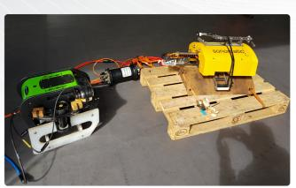
The unit has an auto release mechanism when working with smaller ROV's to enable minimum effort for removal. The unit has an ultrasonic probe head garaging mechanism, for protection during deployment/recovery.
