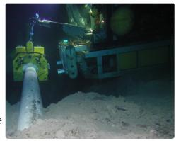
The tools are built around Sonomatic's extensive field experience with challenging subsea inspections and integrate our proven Microplus ultrasonic systems and software with bespoke in-house designed scanner hardware.
