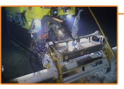
The inspection systems are pressured-rated to 3000m and have been utilised in the field to 1430m water depth to date. Minimal dredging required for 360-degree coverage, (500 mm below pipeline).
