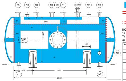
Time of Flight Diffraction inspection for wall loss at weld roots (100% coverage) Time of Flight Diffraction inspection for wall loss at weld roots (Sampling)
