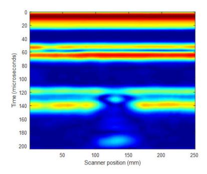
The Sonomatic topside EMAT system uses a pitch-catch setup with one probe acting as a transmitter and another as a receiver. The probes produce shear horizontal (SH) guided waves and provide information on the condition of the sample between the transmitter and receiver. The probes can be separated by over one metre and are sensitive to both internal and external degradation. This system is suitable for material with a thickness range between 3 mm and 15 mm.
