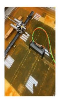
Figure 1: API Qualification Plate and PA MUX System
