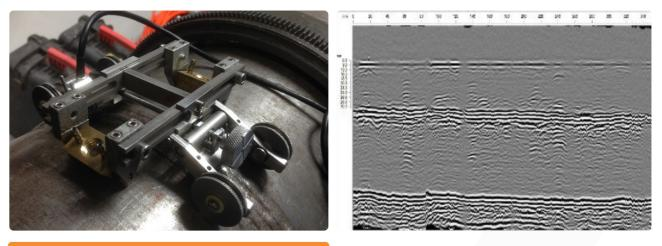
Magnetic wheel based scanner for the inspection of butt welds at temperature up to 400 °C.
