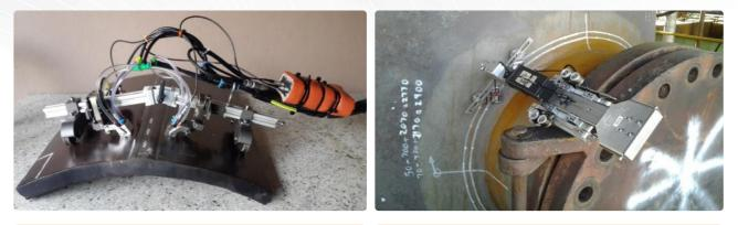
Hinged to accommodate longweld and circweld configurations at temperatures up to 400 °C.
