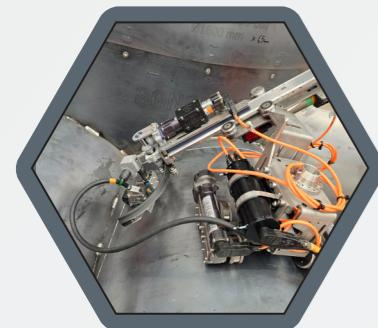
The Node Ray Scanner is designed to overcome the limitations of traditional inspection methods. Its articulating multi-function head allows precise tracking of intricate node geometries, ensuring consistent probe positioning throughout the inspection process.
