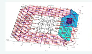
This image shows the model of the tank that was created with the weld layout. Data was uploaded onto the model and could be displayed in different ways, for example the image shows plates coloured by minimum thickness on the plate.
