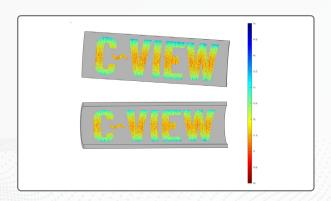
This example creates a thickness map as shown on the left, a further 4 corrosion maps are created which have Sonomatic and C~View text in the composites. These additional maps can be chosen in C-scan selection on the right panel.
