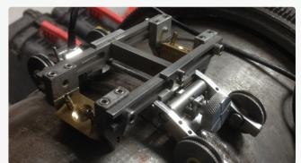
Magnetic wheel based scanner for the inspection of butt welds at temperature up to  $400\,^{\circ}\text{C}$ .
