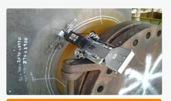
Smaller compact magnetic wheel based scanner to accommodate smaller diameter pipe butt-welds and longwelds at temperatures up to 400 °C.
