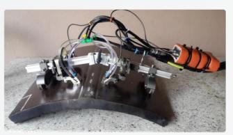
Hinged to accommodate longweld and circweld configurations at temperatures up to 400 °C.
