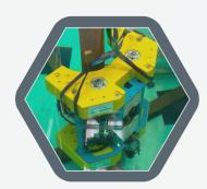
The MEC-Hug™ PipeCrawler is a sophisticated self-crawling inspection system able to scan in both axial and circumferential directions. It has been developed to provide a reliable and technically advanced inspection solution for flexible risers and flexible pipes at their working locations while accommodating the various degrees of wire angle structures.
