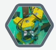
The MEC-Hug<sup>™</sup> PipeCrawler is a sophisticated self-crawling inspection system able to scan in both axial and circumferential directions. It has been developed to provide a reliable and technically advanced inspection solution for flexible risers and flexible pipes at their working locations while accommodating the various degrees of wire angle structures.
