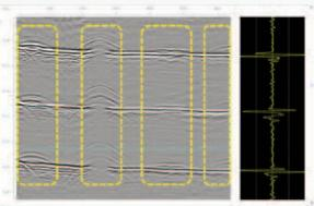
In the case of localised degradation the data is analysed to estimate the depth of flaws. In the case of general degradation the data is analysed to estimate the average remaining wall thickness.
