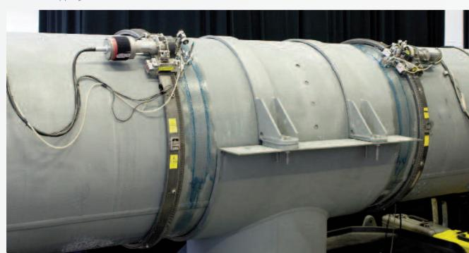
The Multiskip technique uses angled shear waves with two transducers in a pitch-catch mode. The transmitter and receiver can be separated by up to 2 m with full investigation of the material condition between the probes. The data can be collected while scanning at reasonably high speeds, allowing for rapid coverage of large areas.
