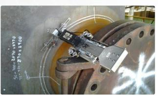
Smaller compact magnetic wheel based scanner to accommodate smaller diameter pipe butt-welds and longwelds at temperatures up to 400 °C.
