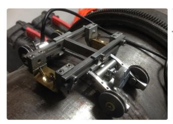
Magnetic wheel based scanner for the inspection of butt welds at temperature up to 400  $^{\circ}\text{C}$ .
