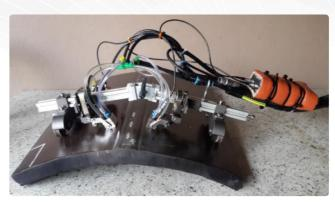
Hinged to accommodate longweld and circweld configurations at temperatures up to 400 °C.
