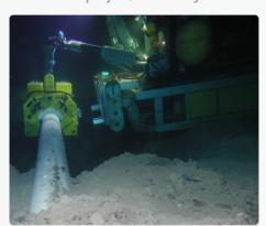
The tools are built around Sonomatic's extensive field experience with challenging subsea inspections and integrate our proven Microplus ultrasonic systems and software with bespoke in-house designed scanner hardware.
