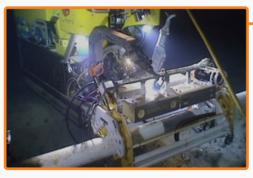
Recent developments allow subsea inspection of concrete weight coated pipelines through the use of subsea Computed Tomography.
