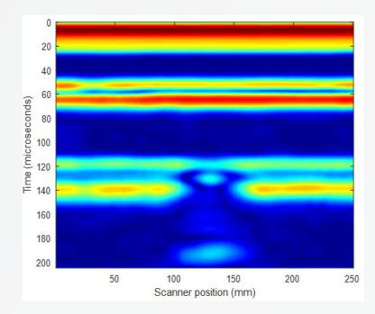
The Sonomatic topside EMAT system uses a pitch-catch setup with one probe acting as a transmitter and another as a receiver. The probes produce shear horizontal (SH) guided waves and provide information on the condition of the sample between the transmitter and receiver. The probes can be separated by over one metre and are sensitive to both internal and external degradation. This system is suitable for material with a thickness range between 3 mm and 15 mm.
