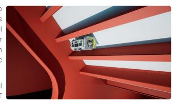
In June 2023, Geo Oceans carried out the first implementation of the i-COT fitted with the Sonomatic Multiplexer UTM probe to take measurements from the water ballast tank walls shared with the crude oil tank on a FPSO based in the Gulf of Mexico to identify the condition of the plate.
