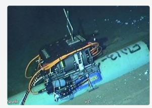
Sonomatic's Subsea MAG-ST crawler has been utilised for both subsea and topside applications and is deployed by an ROV onto the region of interest. The crawler is fixed to the pipe using permanent magnetic wheels, and its position can be recorded by onboard encoders and inclinometers to record positional feedback, whilst progress can be monitored using attached cameras.
