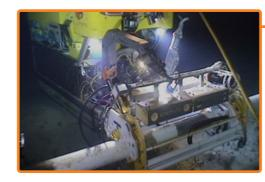
Recent developments allow subsea inspection of concrete weight coated pipelines through the use of subsea Computed Tomography.
