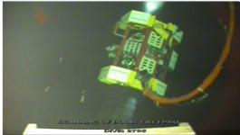
Report extraction: signal consistent with increased wire gap of the order of 5-10mm. No cracks/metal loss/corrosion.
